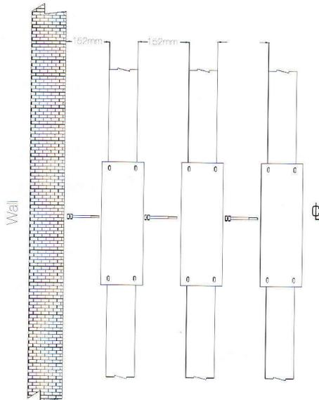
In case the busway been installed side by side.
